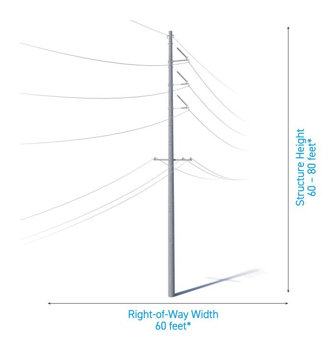
Most of the existing line consists of wooden poles. Crews plan to rebuild the line using a majority of steel single-pole structures. At select points, crews plan to use concrete single-pole structures. Proposed Structures area an average of 20 feet taller than the existing structures.
