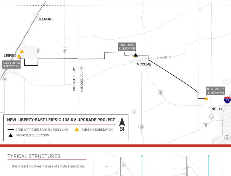
Typical Pole Height Range: 75-95 feet\* Typical Right-of-Way Width: 100 feet\*
