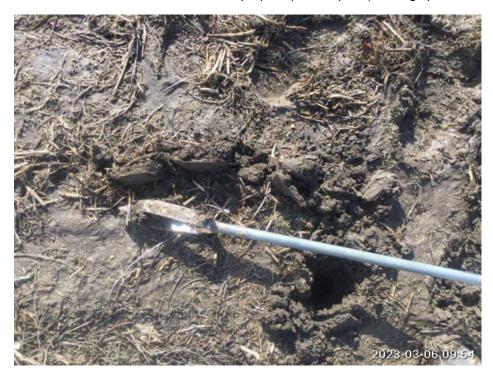
Photo Location 1. View of wetland determination sample point (SP02: upland), soil profile.
